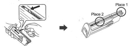
pull the spring lever back and load the BBs
